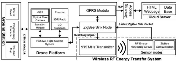
Figure 1: System architecture.
