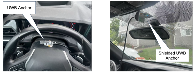
(a) Anchor on top of steering wheel. (b) Anchor next to rearview mirror with a shield attached.
