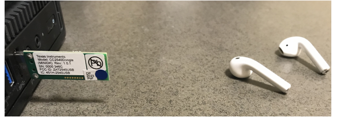
Figure 1: BBC enables direct communication between BLE chips and Bluetooth-Classic headphones
