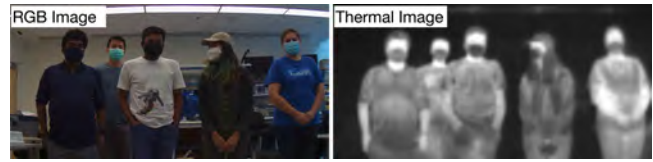
Figure 2: The Lepton 3.5 thermal camera measures black body radiation (long wavelength IR) to provide an absolute measure of surface temperature. This permits robust operation across various skin tones, body shapes, and genders.
