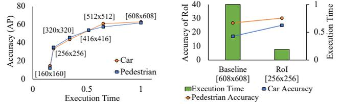
(a) Comparison of execution time and (b) Comparison of accuracy of RoI accuracy by down-sampling.
