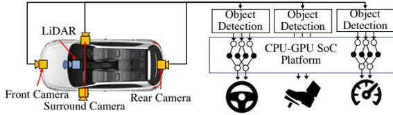
Fig. 1. An example of DNN-based object detection systems
