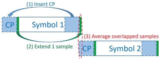
Figure 2: CP insertion and OFDM symbol windowing
