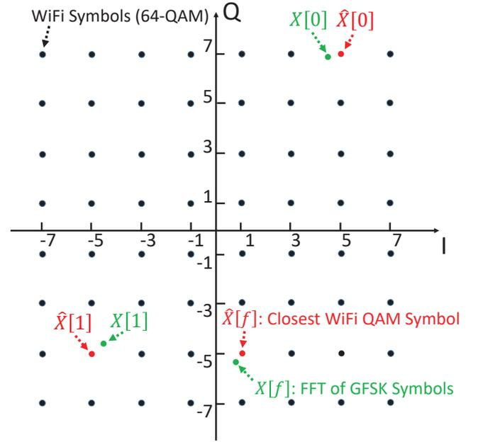
**Figure 4: Selecting  $\hat{X}[f]$  from  $X[f]$ .  $X[f] = FFT(x[n])$ . A scale factor  $A$  is applied ( $x[n] = A \cdot e^{i \cdot \phi[n]}$ ) so that  $X[f]$  is appropriately scaled w.r.t. origin.**
