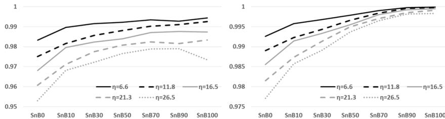
Fig. 10. (left) Cumulative percentage of update delay is  $\leq 100$ ms for different densities (20ms broadcast); (right) Cumulative percentage of update delay is  $\leq 200$ ms for different densities (20ms broadcast)
