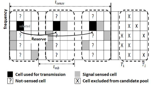
Fig. 1. Sensing-based semi-persistent scheduling ( $T_1 = 2, T_2 = 5$ )
