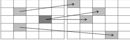
Fig. 5. (Left) Two vehicles use same subframe in column 2. Two vehicles use same resource in column 4. (Right) Resolving CMRFs via random selection.
