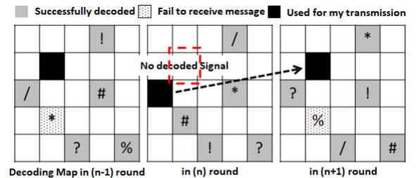
Fig. 6. Example of Shake and Back
