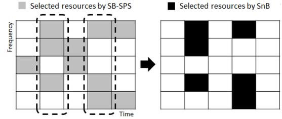
Fig. 4. (Left) Selected resources by SB-SPS; (Right) Final resource candidates selected after filtering out resources in non-least-used subframes
