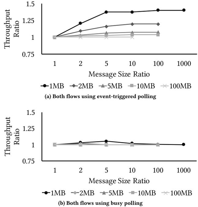
**Figure 4: Ratio of bandwidth allocations of two elephant flows for increasing gaps between their message sizes for varying base flow sizes (1MB to 100MB).**
