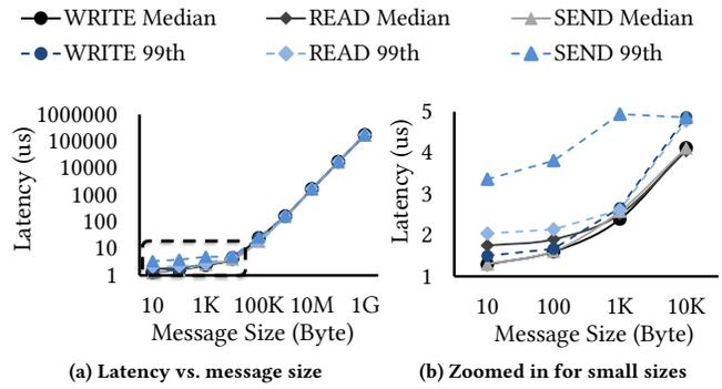
**Figure 1: Median latencies for different RDMA verbs and message sizes.**
