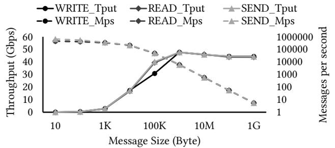
**Figure 2: Throughput in terms of bandwidth (for elephants) and messages per second (for mice) for different RDMA verbs and message sizes.**
