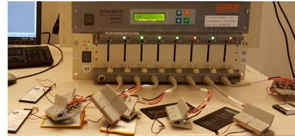
**Figure 11: Laboratory settings for cycling tests.**
