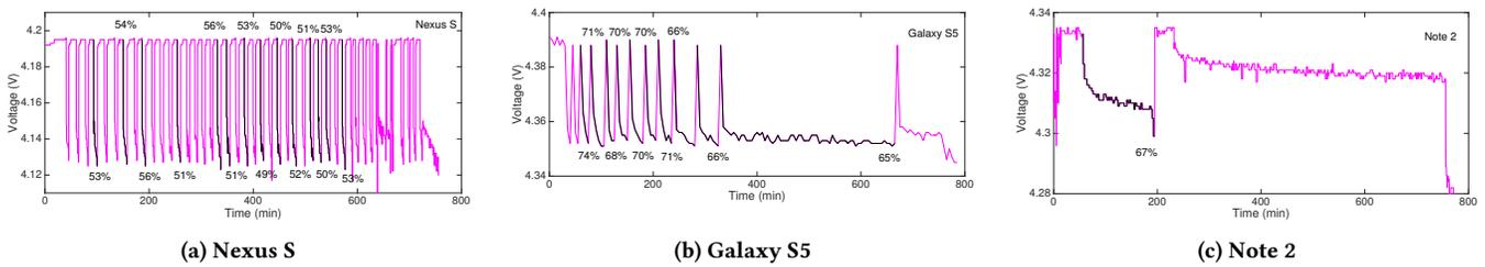
**Figure 18: Field-tests results of V-BASH on Android devices: (a) 14 valid relaxing sub-traces are extracted on Nexus S, concluding a (estimated) mean SoH of 52%; the measured true SoH is 54.9%; (b) 10 valid relaxing sub-traces are extracted on Galaxy S5, concluding a (estimated) mean SoH of 69%; the measured true SoH is 74.2%; (c) 1 valid relaxing sub-trace is extracted on Note 2, concluding an estimated SoH of 67%; the measured true SoH is 73%.**
