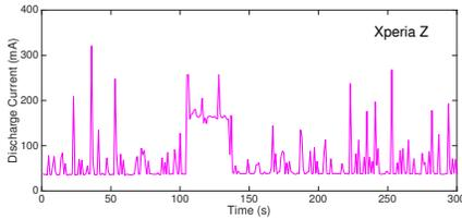
**Figure 8: Battery is continuously discharged even for idle devices.**
