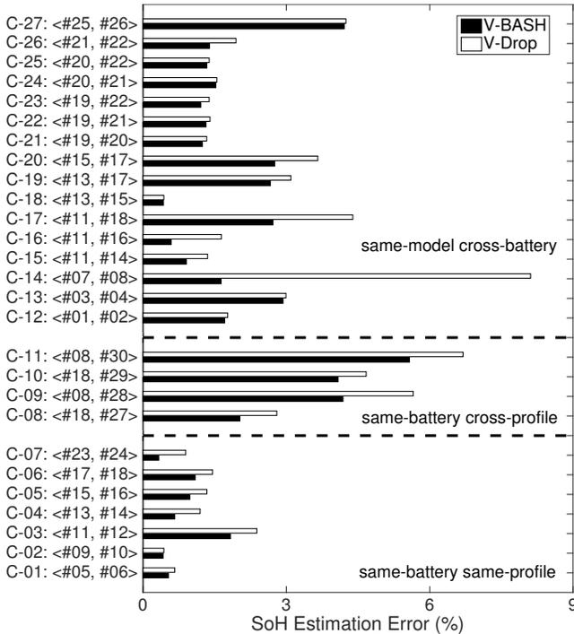
**Figure 16: Evaluation of V-BASH with laboratory experiments: (bottom) V-BASH is trained and validated based on traces collected with the same battery during different tests with identical profiles; (middle) V-BASH is trained and validated based on traces collected with the same battery during tests with different profiles; (top) V-BASH is trained and validated based on traces collected with different same-model batteries.**
