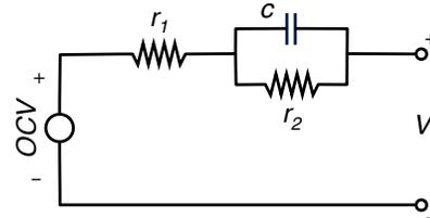
**Figure 7: Thevenin’s battery circuit model, consisting of a series resistor and a parallel resistor-capacitor.**
