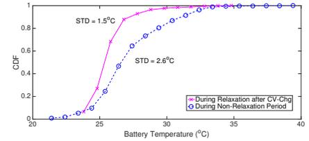
**Figure 10: More stable battery temperature during after-charging relaxation.**
