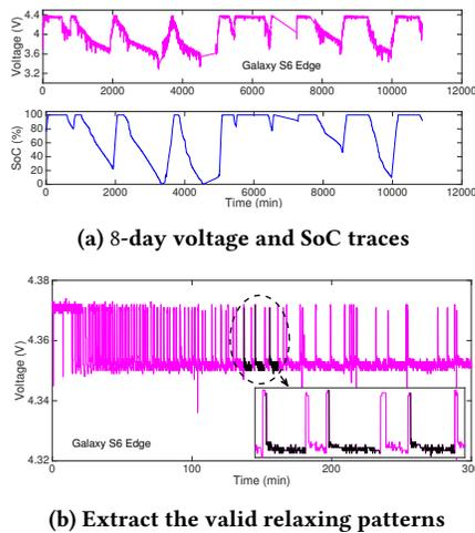
**Figure 17: Collecting the relaxing voltage traces of a Galaxy S6 Edge phone: (a) the collected 8-day traces; (b) extracting valid relaxing patterns from trickle-charging-polluted traces (zoom-in of the first 500 minutes voltage traces of (a), during which the phone has 100% SoC).**
