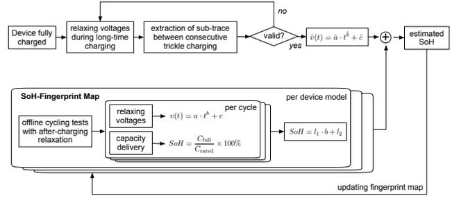
**Figure 15: V-BASH overview: the device collects its relaxing voltages, which are compared with the offline constructed fingerprint map for SoH estimation. Thus-estimated SoH is then used to update the fingerprint map.**
