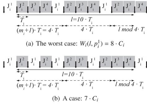
**Fig. 3.** The amount of execution of  $\tau_i$ 's jobs with priority higher than  $p_i^1$  in an interval of length  $l$  such that the interval starts at one of the release times of jobs of  $\tau_i$ .
