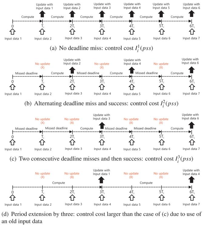
Fig. 2. Control cost by different update frequencies, where Update  $i$  is the output computed using Input data  $i$ .
