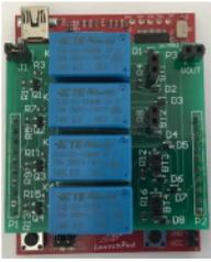
Fig. 17. Reconfigurable battery board prototype.
