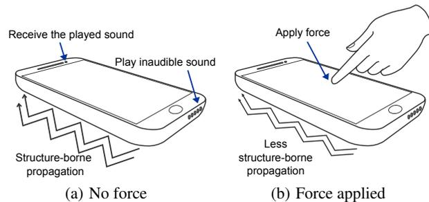
**Figure 1—Structure-borne propagation and the applied force.** When no force is applied to the phone, the frame and internal components of the phone can vibrate freely, and hence the played inaudible sound can easily propagate through the phone's body.
