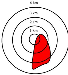
Figure 1: Each scan partitions the candidate area into a group of concentric rings and keeps one of them.
