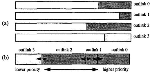
**Figure 6. (a) Sorted entries in separate priority queue showing wasted resources; (b) Same entries in the multiple shift register priority queue**
