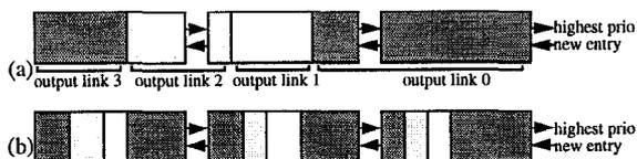
**Figure 9. Storage of entries in the multiple systolic array queue (a) before and (b) after “atleast-1-entry-per-outputlink” property**
