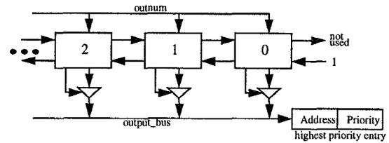
**Figure 7. Multiple shift register priority queue**
