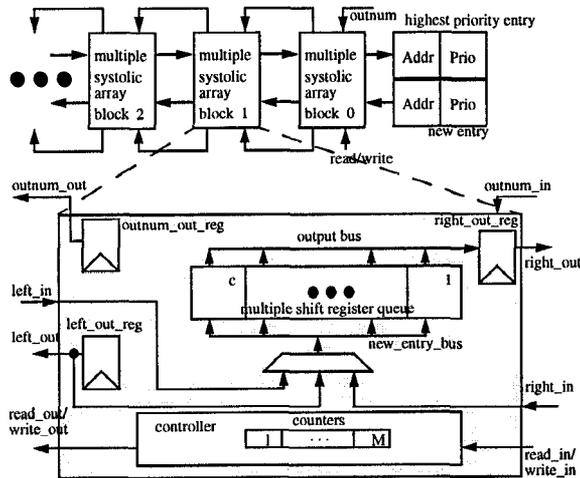
**Figure 8. Multiple systolic array priority queue and block**
