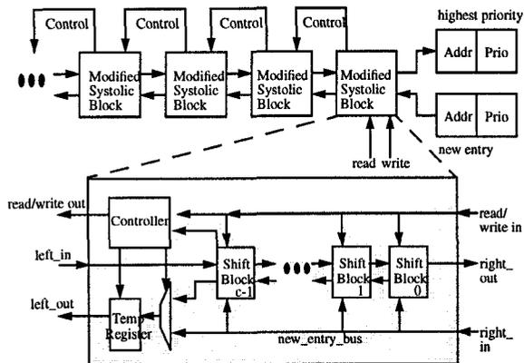
**Figure 4. Modified systolic array priority queue**
