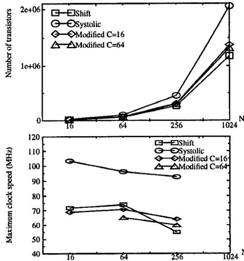
**Figure 12. Modified systolic architecture results compared to that of the shift and systolic.**
