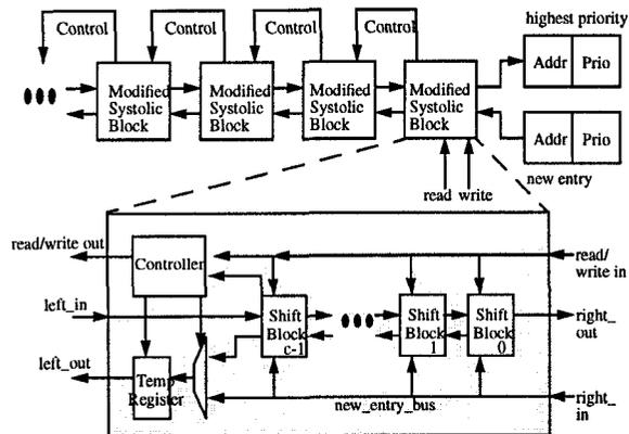
**Figure 4. Modified systolic array priority queue**
