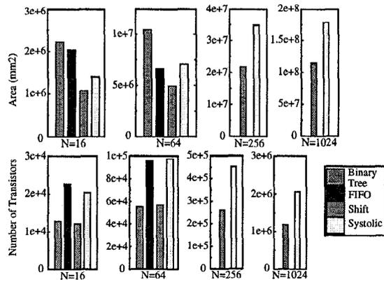
Figure 10. Implementation results for existing priority queue architectures (P=16).
