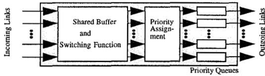
**Figure 1. Simplified block diagram of a single shared buffer switch architecture with link scheduling**
