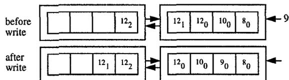
**Figure 5. Data movement in the modified systolic array PQ showing a potential ordering problem**
