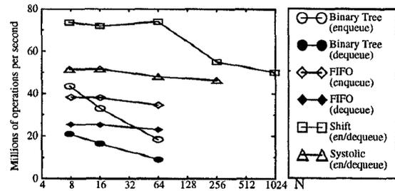
Figure 11. Scaling effects on performance as N increases (P=16)
