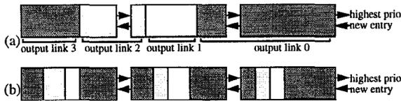
**Figure 9. Storage of entries in the multiple systolic array queue (a) before and (b) after “atleast-1-entry-per-outputlink” property**
