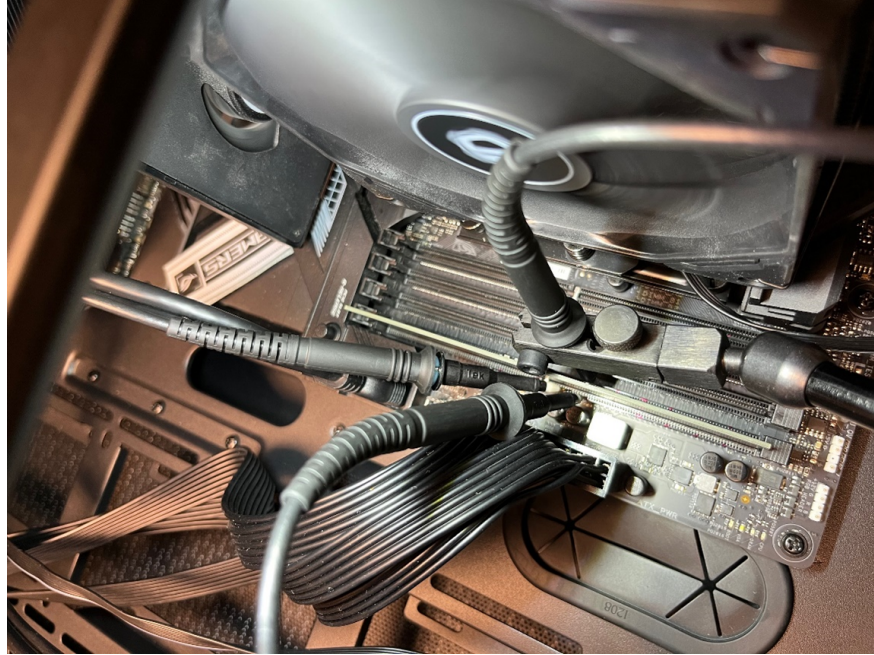
Figure 2.2: Physical probing experimental setup.
