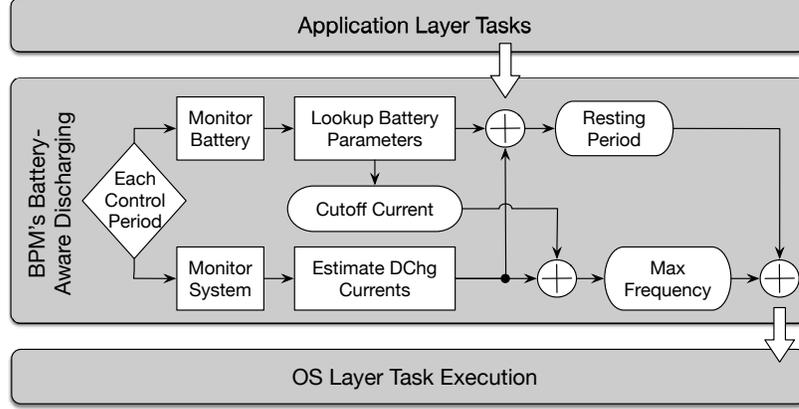
Figure 2.18: Control flow of BPM's battery-aware discharging management.
