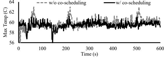
Figure 5.9: Transient temperatures w/o and w/ CPU–GPU co-scheduling.
