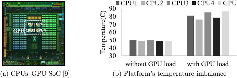
Figure 5.2: CPUs surrounded by the GPU cluster on a SoC (Tegra X1), where the GPU’s power dissipation affects the CPUs’ temperatures, creating temperature imbalance across the CPUs.
