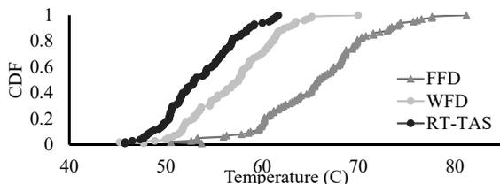
Figure 5.11: Maximum temperature CDF for different task sets.
