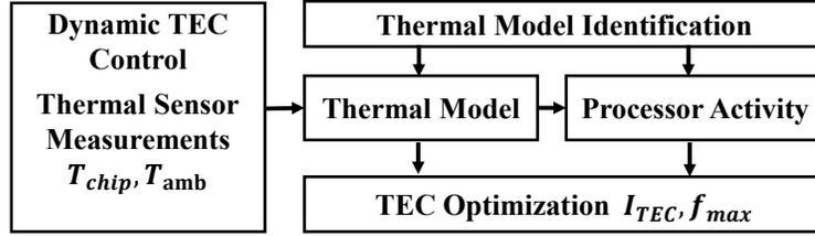
Figure 3.7: Workflow diagram of dynamic TEC control.
