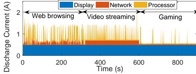
Figure 2.14: The processor incurs a burstier discharge current than other components.
