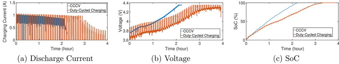
Figure 2.10: BPM’s duty-cycled charging vs. standard CCCV charging.
