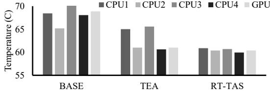
Figure 5.7: Core-level peak temperature under different scheduling policies.
