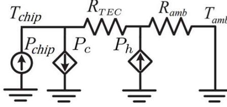
Figure 3.4: Thermal circuit model of the TEC system.
