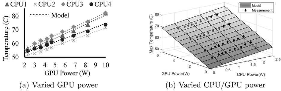
Figure 5.4: (a) CPU temperatures resulting from varied GPU power dissipations and (b) maximum CPU temperature resulting from varied CPU and GPU power dissipations.
