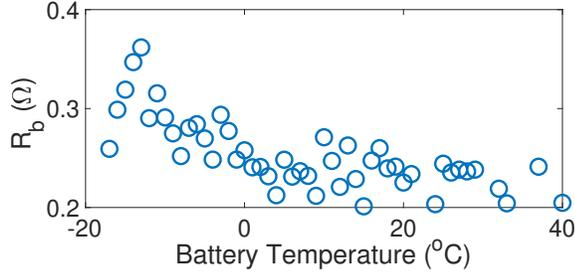
Figure 2.5: Battery impedance rises as temperature falls.
