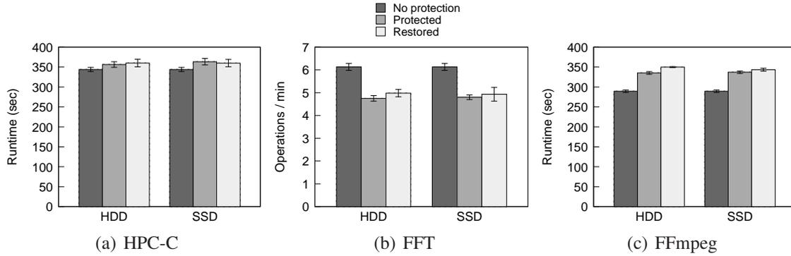
Figure 3.5: The performance of the workloads under different conditions: *no protection* and not checkpointed, *protected* and configured to be checkpointed every second, and *restored* from a failure that occurs halfway through the workload executions.
