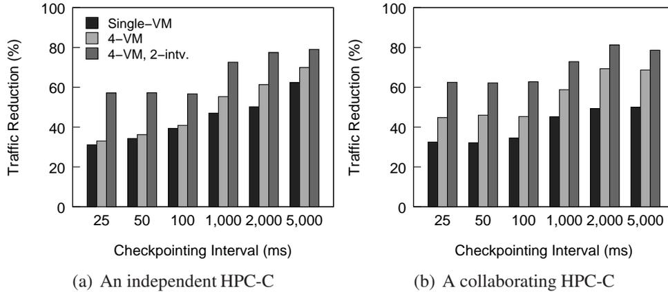
Figure 2.3: The traffic reductions achieved by similarity compression for a HPC-C VM when the VM’s checkpoints are processed alone (Single-VM), together with other VMs’ checkpoints in a 4-VM HPC cluster (4-VM), and using a two-interval hash table (4-VM, 2-intv.)
