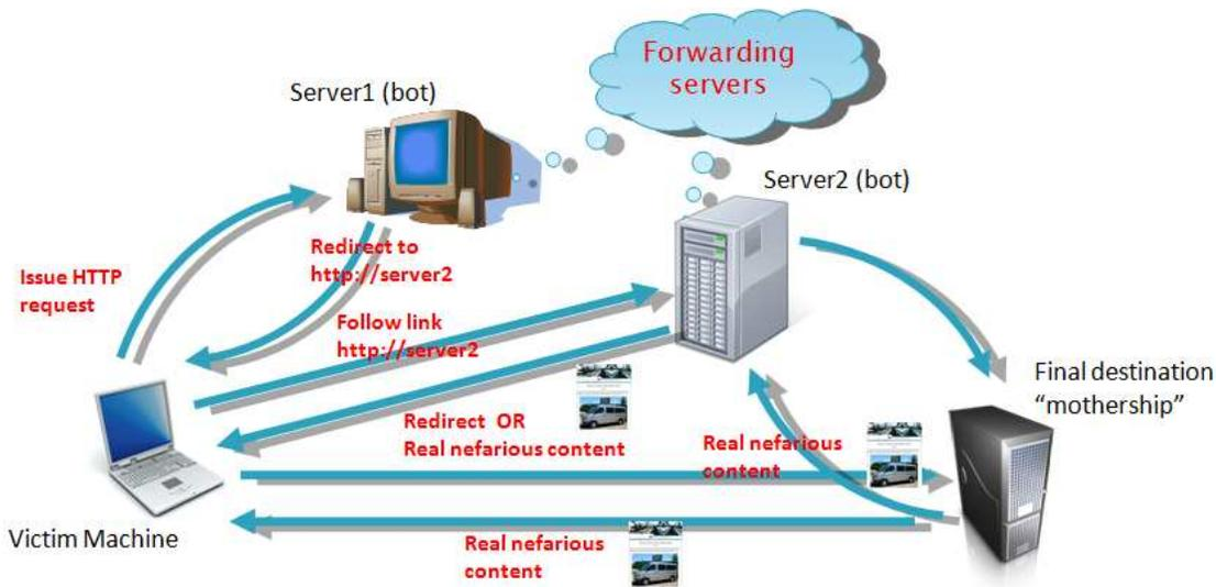
Figure 1.1: Fast-Flux botnet redirection/proxy mechanism
