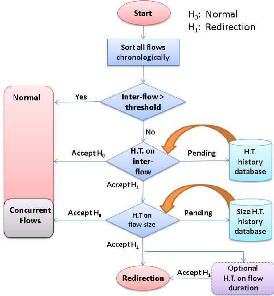
Figure 2.2: Flowchart of the algorithm for identification of redirection behaviors
