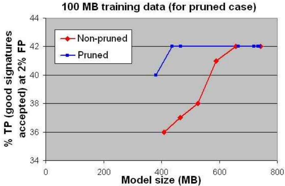
Figure 4.2: TP rate comparison between pruned models and non-pruned models when the training set varies from 50 Mbytes to 100 Mbytes
