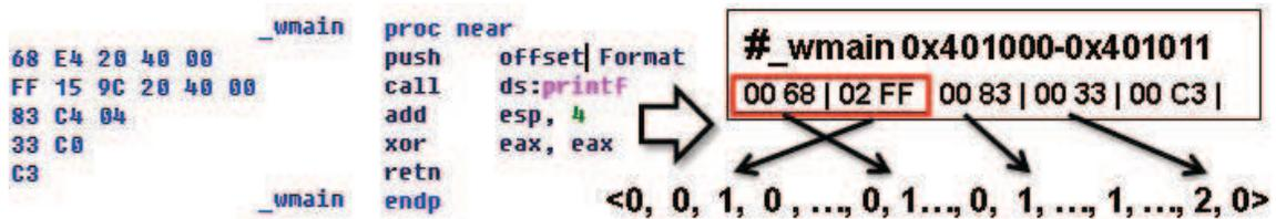
Figure 3.4: Encoding a function into a standardized format
