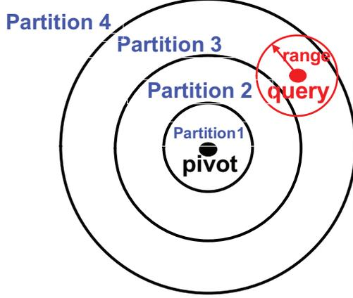
Figure 2.4: Pruning on a VPT based on the triangular inequality
