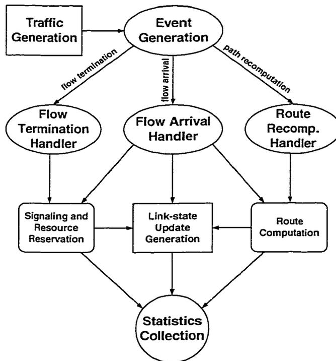
Figure 3.2: routesim functional components
