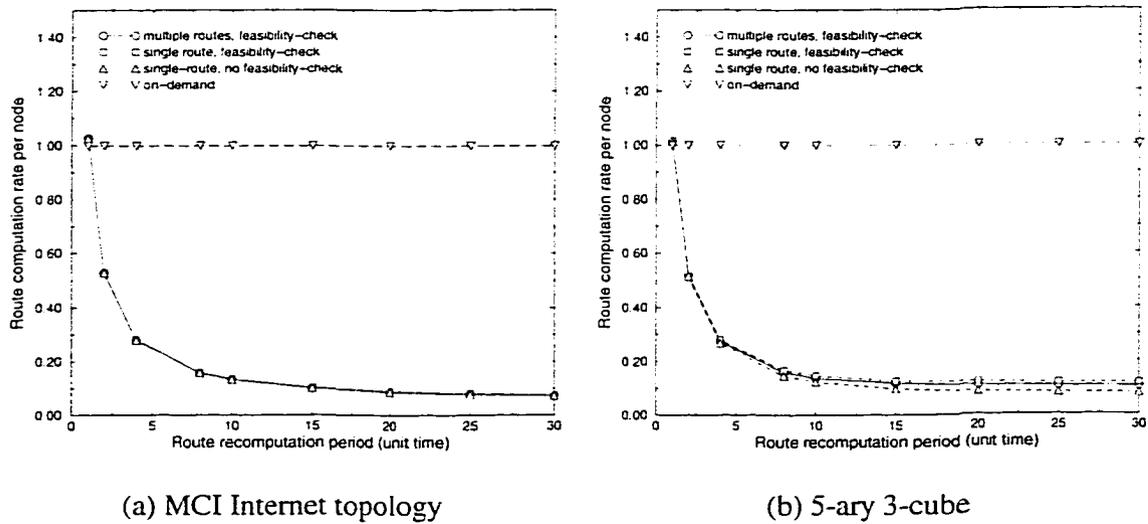
**Figure 5.6: Overhead with accurate link state**
