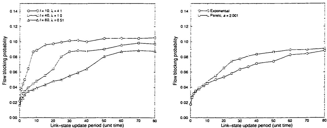
(a) Blocking for different mean durations      (b) Blocking for different distributions ( $\ell = 40$ )
