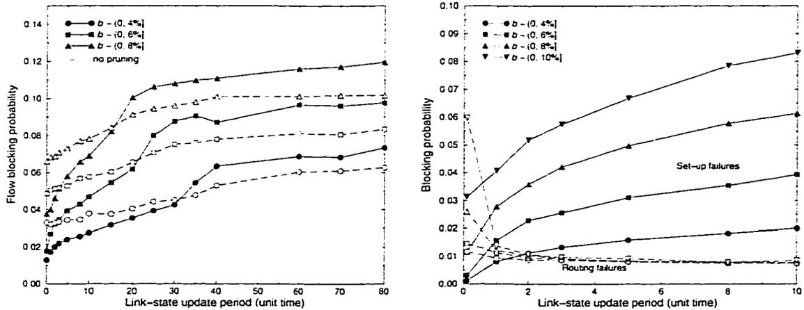
(a) Flow blocking vs. update period (b) Routing and set-up failures (with pruning)
